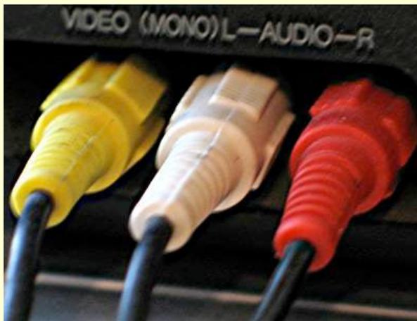
Three color-coded RCA cables plug in to a composite video port.
