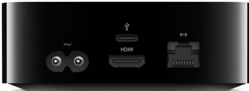
**Figure 1:** Fourth-generation Apple TV ports, from left to right: power, USB-C, HDMI, and 10/100 Ethernet.
