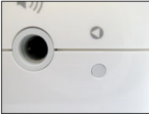
Figure 1: The reset button is located below the reversed-out white arrow; here, it's next to the audio port of an AirPort Express.
