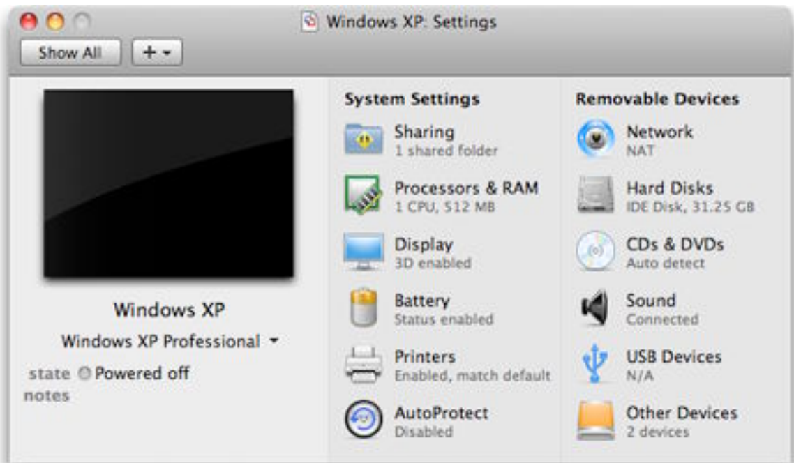
Figure 11: The Settings window. Click a category to configure its settings for the selected virtual machine.
