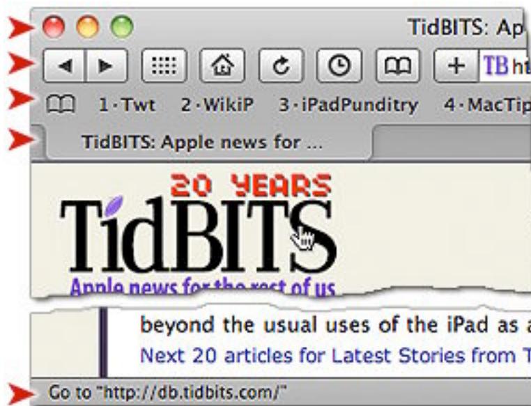
Figure 1: The top "bars" don't look separate, but different areas provide different functionality. From top to bottom: the title bar, the toolbar, the bookmarks bar, the tab bar, and the status bar.
