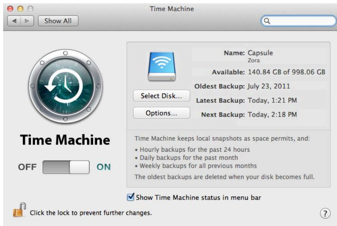
Figure 7: Specify backup drives and ignored volumes in the Time Machine preference pane.
